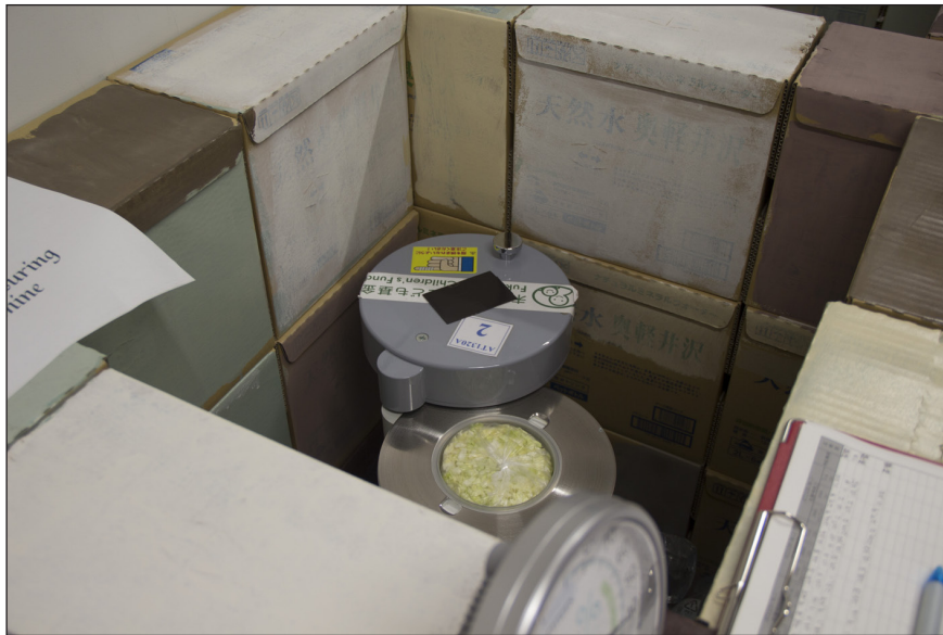
Figure 9: Radiometer measuring the radiation levels in local cabbage at Tarachine in Iwaki, Fukushima. Photo courtesy of Hayat Rasul.
